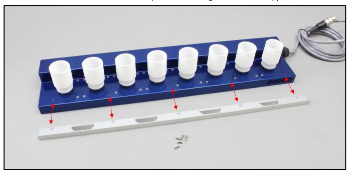
3. Make sure the trapezoidal holes in the Support Rail have the short side to the outside, away from the Spin Bases.
